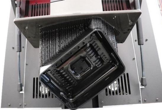
Bottom cover of an electronic housing part in the size 144x40x114 mm 3D printed on Asiga Pro 4k with Henkel's Loctite 3843
